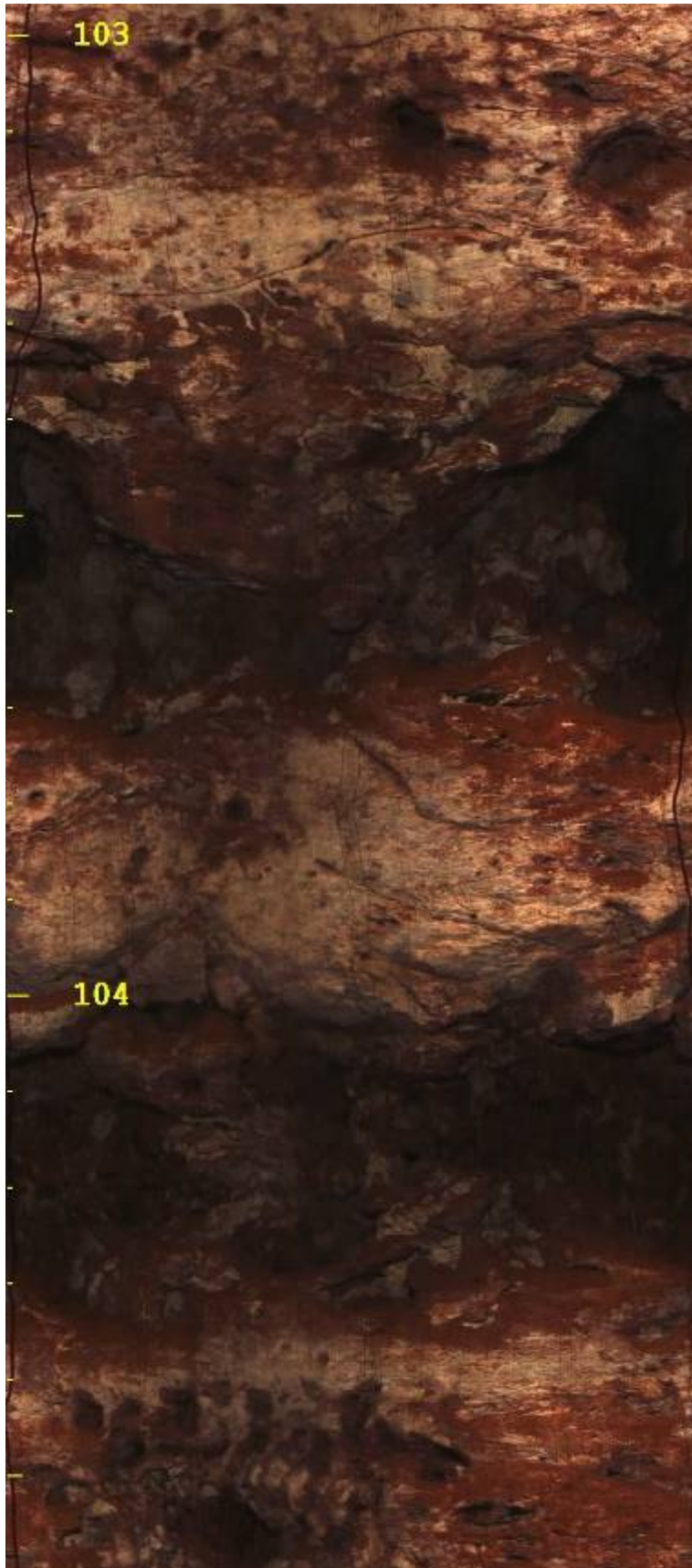
Plate 1 RN37042, 103 – 104.6m, down-hole optical scanner image
