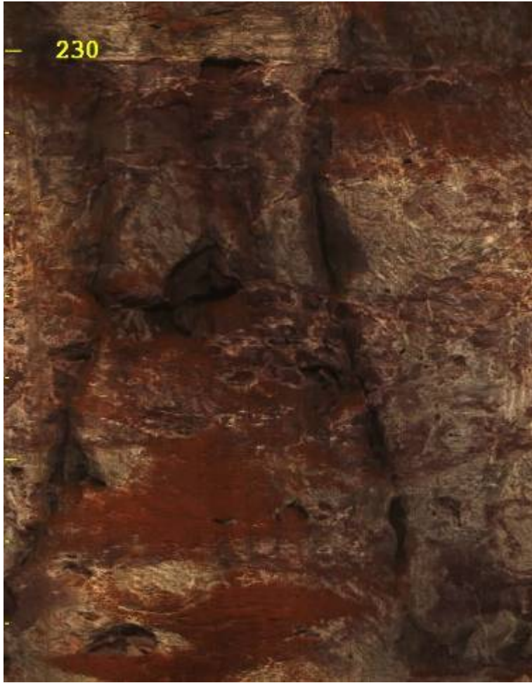
Plate 8 RN37043, 230 – 230.8m, down-hole optical scanner image
