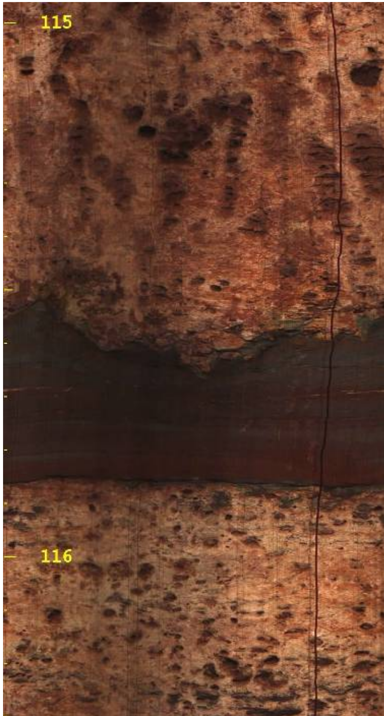
Plate 2 RN37042, 115 – 116.3m, down-hole optical scanner image
