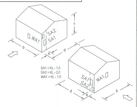
**ROOF - LOCAL PRESSURE ZONES** NOTE - "a" = The lesser of 0.2b, 0.2d & h "h" = Average Structure Height
